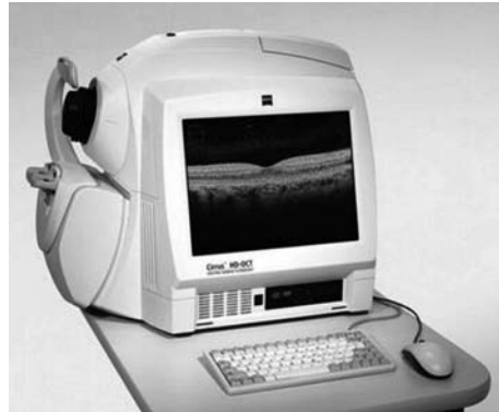
The Cirrus Spectral Domain Optical Coherence Tomography (OCT)
